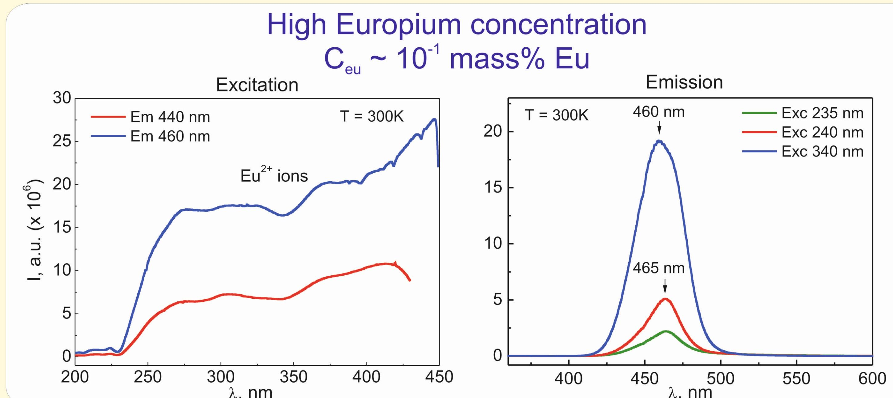
Several emission bands connected with different types of centers are found in CsI:Eu crystals excited in range of typical absorption bands at RT. Intensity and spectra of luminescence depend on activator' concentration. The strong overlapping of absorption and emission spectra for high concentrated crystals are present, which leads to self-absorption.
