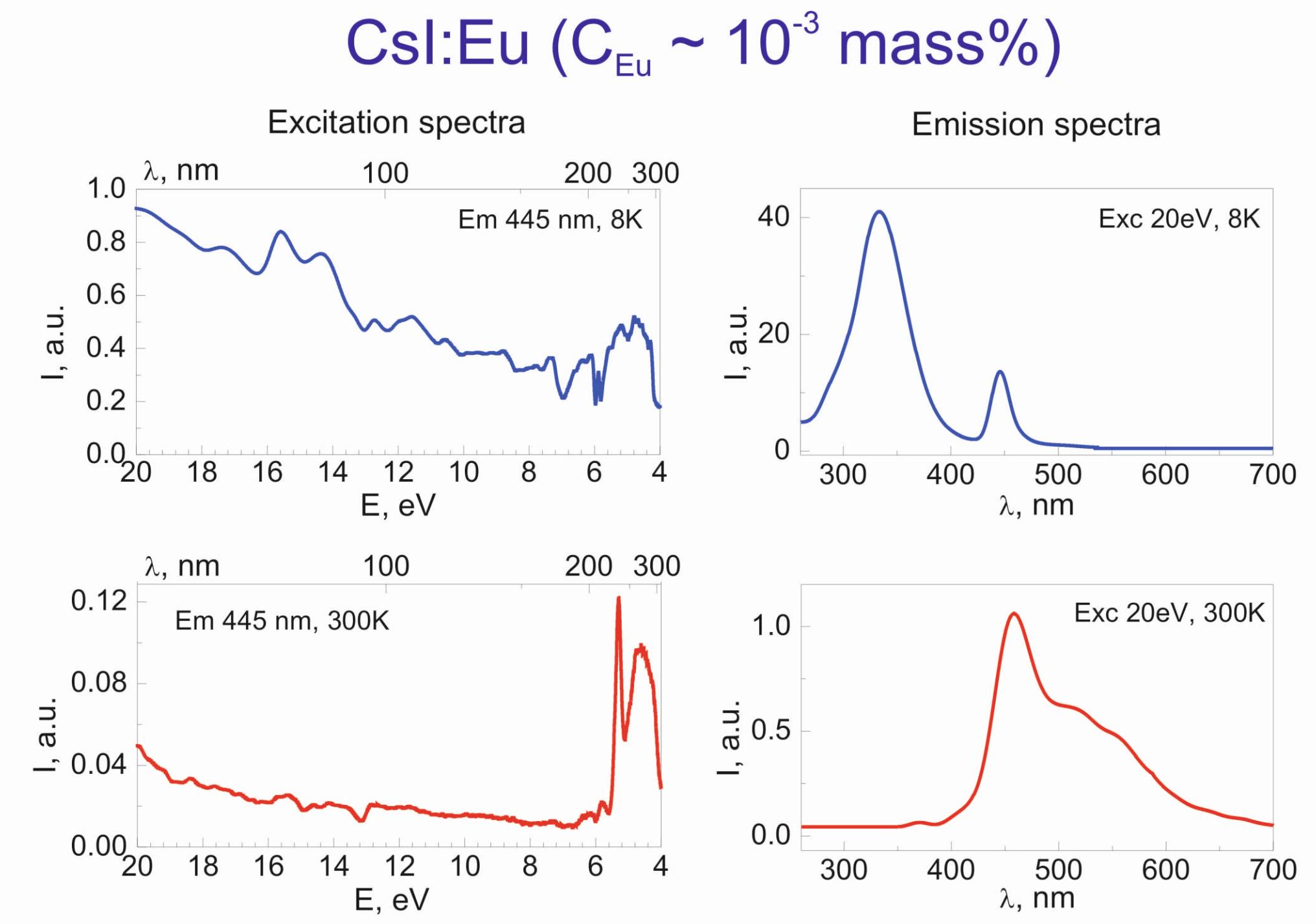
Spectral studies performed upon the synchrotron excitation within 4-20 eV range at 8-350K show that favorable conditions have been revealed for the transformation of VUV excitation quanta into Eu<sup>2+</sup> emission at low temperatures (<150 K). In this region the main intense band is π-STE luminescence peak at 340 nm. An addition one at 456 nm corresponds to Eu<sup>2+</sup> emission.
