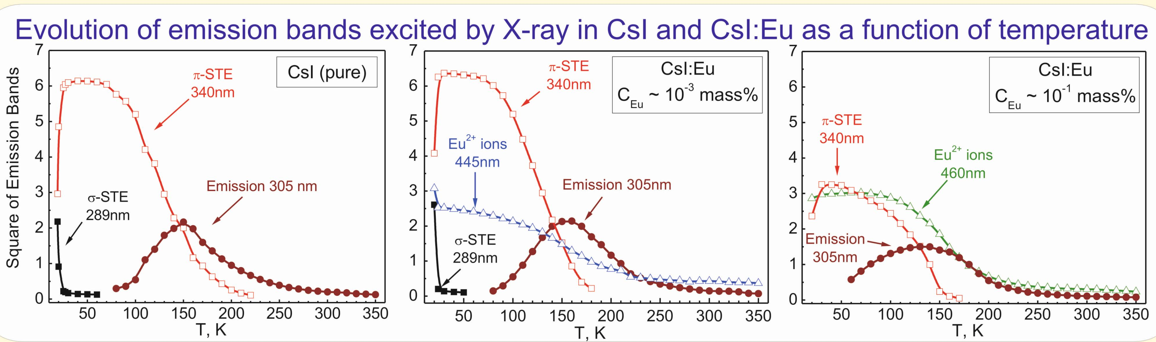
Excitation of CsI:Eu crystals by X-ray at RT leads to appearance of intrinsic band (305nm) and addition peaks at 410 and 445 nm in luminescence spectra of slightly doped crystal, whereas intense 460 nm band is found in highly doped sample.
